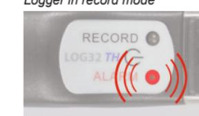
Beeper sounds once each 30 seconds for 1 second, red LED blinks each 3 seconds - measured values exceeds selected measurement range (not with standard settings). Alarm limits can be changed using LogConnect\* software.
