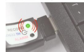
Connect logger to USB port. Beeper sounds for 1 second. LED blinks green until result PDF is created (can take up to 40 seconds).
